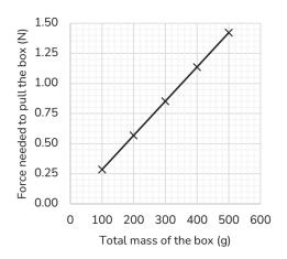
b) The force needed to pull the box is equal in magnitude to the frictional force  $F_f$  on the box:  $F_f = \mu N = \mu mg = \mu \times 9.8 \times \text{mass in grams} \div 1000$  As  $F_f$  is plotted on the y-axis and mass in grams on the x-axis, the gradient =  $\mu \times 0.0098 = 0.0028$  from the graph. So the coefficient of friction  $\mu$  is 0.29.
